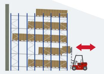
The pallet is introduced in the loading aisle and by gravity it slides over the rollers to the opposite side, where the unloading aisle is located.
