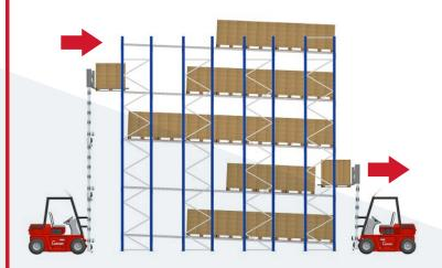
The pallet is introduced in the loading aisle and by gravity it slides over the rollers to the opposite side, where the unloading aisle is located.
